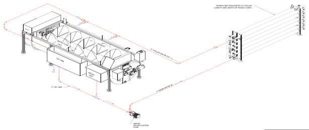
The CIP tank must be filled with enough hot soapy water to clean the entire run of tubing. Industry standard is to size the CIP tank at least 15% more than the volume of the tubing so that there will be some water left in the tank after the tubes are filled. What size CIP tank should you put on the machine? If the height of the tank is 3', recommend CIP tanks with 2 different sets of dimensions.
